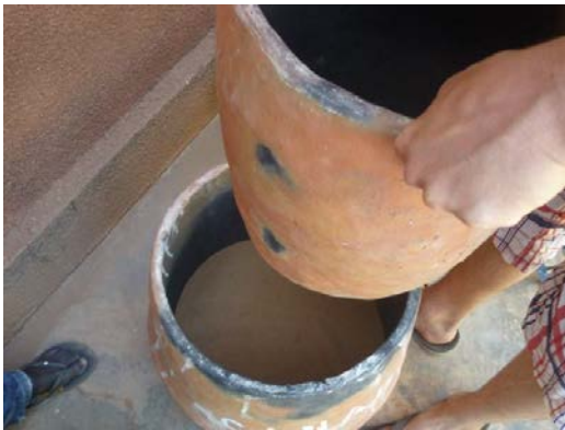
Figure 7: Smaller clay pot is placed in the bigger clay pot.
