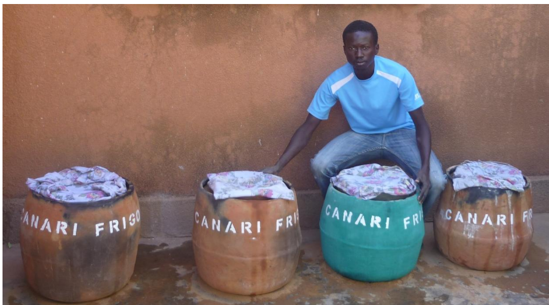
Figure 10: Movement team member with a test series of four covered clay pot coolers
